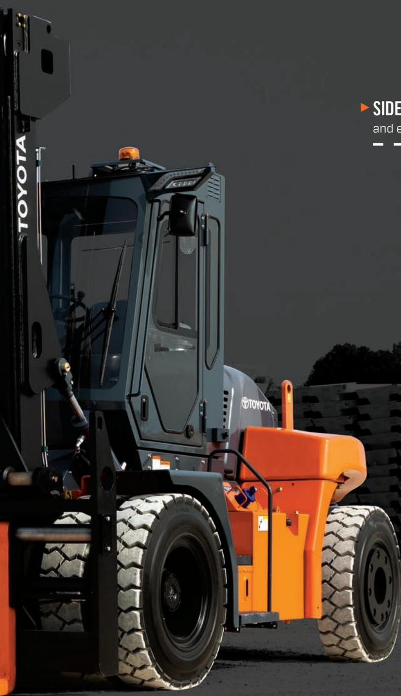
▶ **SIDE-TILT CAB** opens 65° for easy access and enhanced serviceability.
